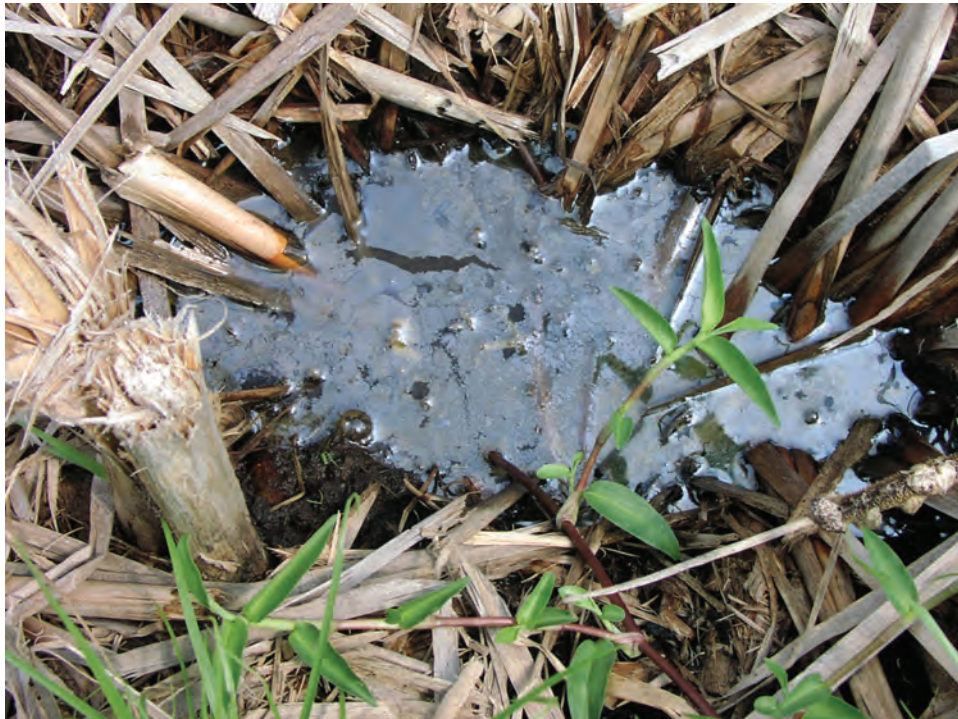
Figure 35. Iron sheen on the water surface may be deposited as an orange or yellow crust after dewatering.
