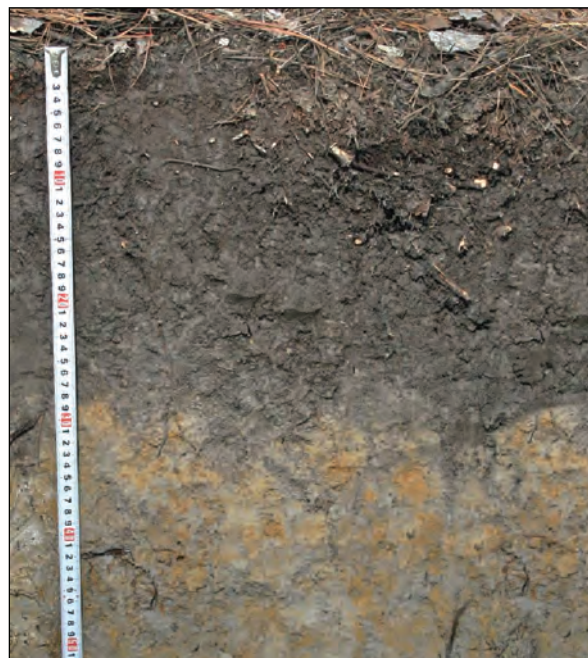
Figure 11. In this soil, a depleted matrix starts immediately below the black surface layer at approximately 11 in. (28 cm). Scale is in centimeters.
