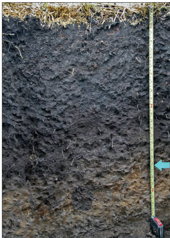
Figure 12. Deep observations may be necessary to identify the depleted or gleyed matrix below a thick, dark surface layer. In this example, the depleted matrix starts at 20 in. (50 cm) (arrow).
