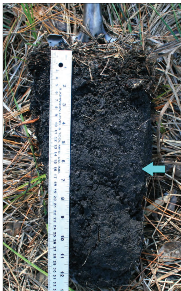
Figure 15. This sandy soil has a dark surface approximately 6 in. (15 cm) thick (bottom indicated by the arrow). Scale is in inches on the right side of the ruler.
