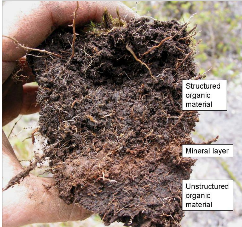
Figure 5. A soil sample from the island of Hawai‘i containing structured (subangular blocky) sapric material at the surface and unstructured (homogeneous) sapric material below. Only the unstructured sapric material (muck) indicates soil saturation.
