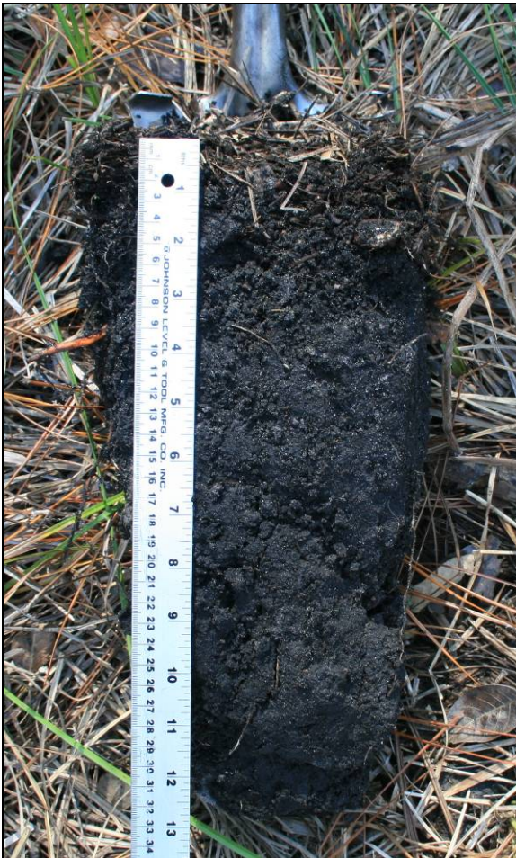
Figure 16. This sandy soil has a dark surface approximately 6 in. (15 cm) thick. Scale is in inches on the right.
