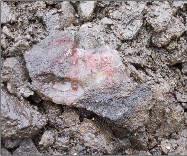
Figure 50. When alpha, alpha-dipyridyl dye is applied to a soil containing reduced iron, a positive reaction is indicated by a pink or red coloration to the treated area.
