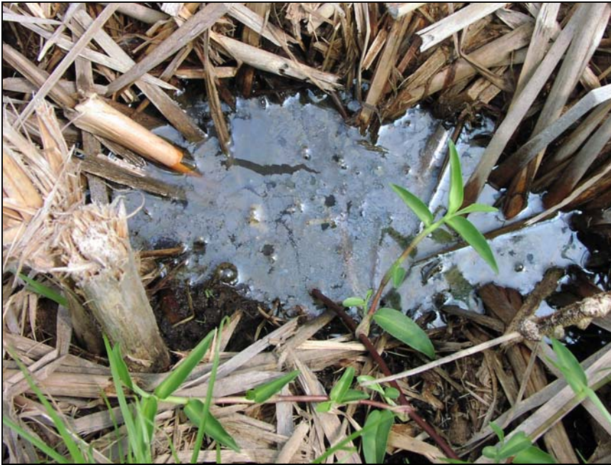
Figure 35. Iron sheen on the water surface may be deposited as an orange or yellow crust after dewatering.
