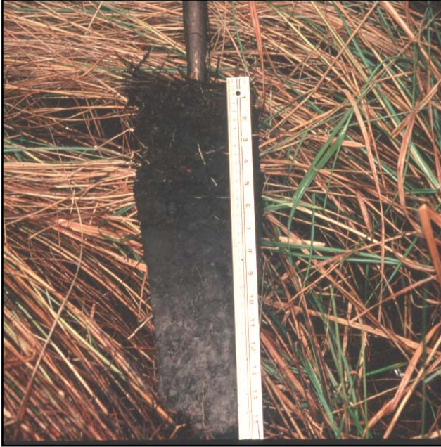
Figure 25. The mucky modified sandy layer is approximately 3 in. (7.5 cm) thick. Scale in inches on the right side of ruler.
