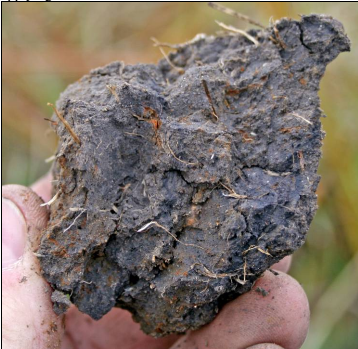
Figure 20. Redox features can be small and difficult to see within a dark soil layer.
