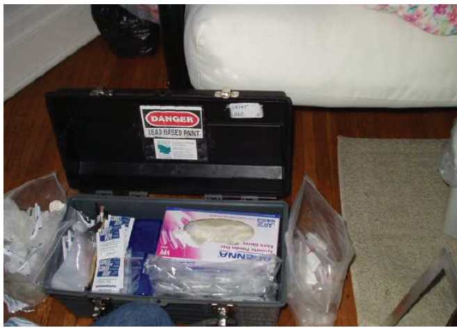
FIGURE 5.11a Dust sampling equipment.
