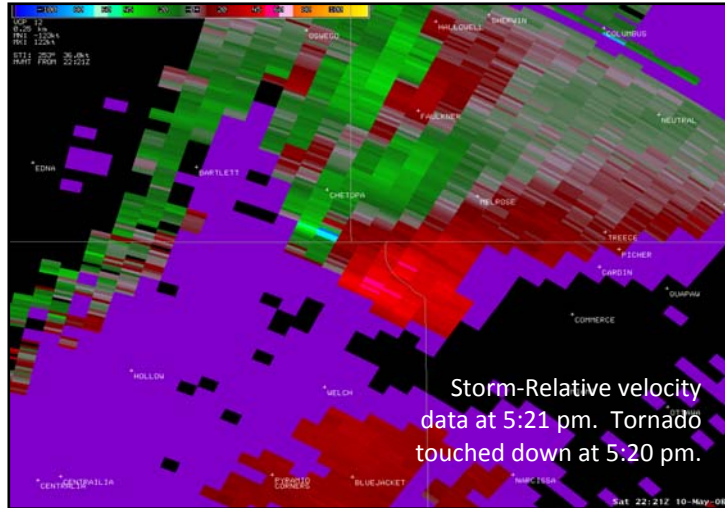
Figure 5. From WFO Tulsa, Oklahoma, Weather Surveillance Radar (WSR-88D), Storm Relative Velocity map at 0.5 degree elevation at 5:21 p.m. The opposing colors of red and green indicate air moving away from the radar (red) and toward the radar (green). Areas where red and green are coupled indicate rotation within a thunderstorm, which often precedes a tornado. The radar is located to the lower left in this image.
