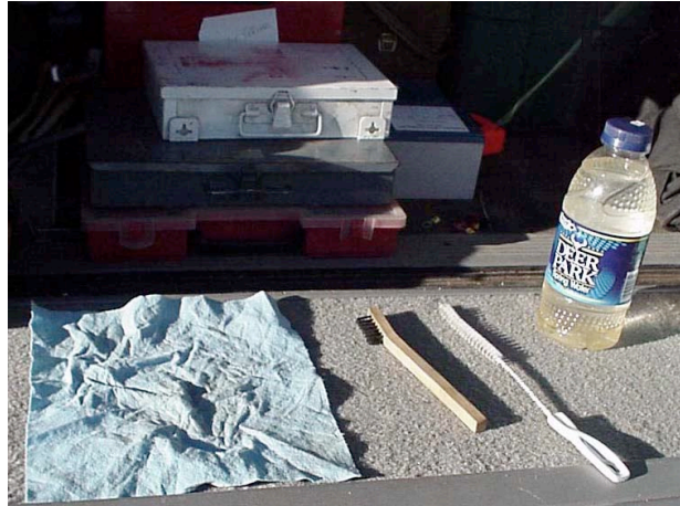
Figure F-3. Cleaning tools: paper shop cloth, teflon mini-brush, bottle brush, water.
