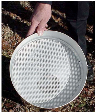
Figure F- 13. Clean screen, top view.
