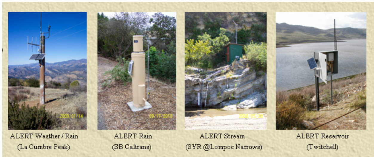
Types of automated (ALERT) flood warning system sensors | Photo: countyofsb.org
