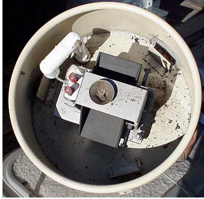
Figure F- 8. Clogged tipping bucket, top view.
