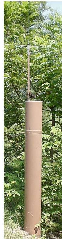
Figure 1-1. Automatic rain gage.
