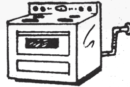
20. gas stove with rigid feed line
