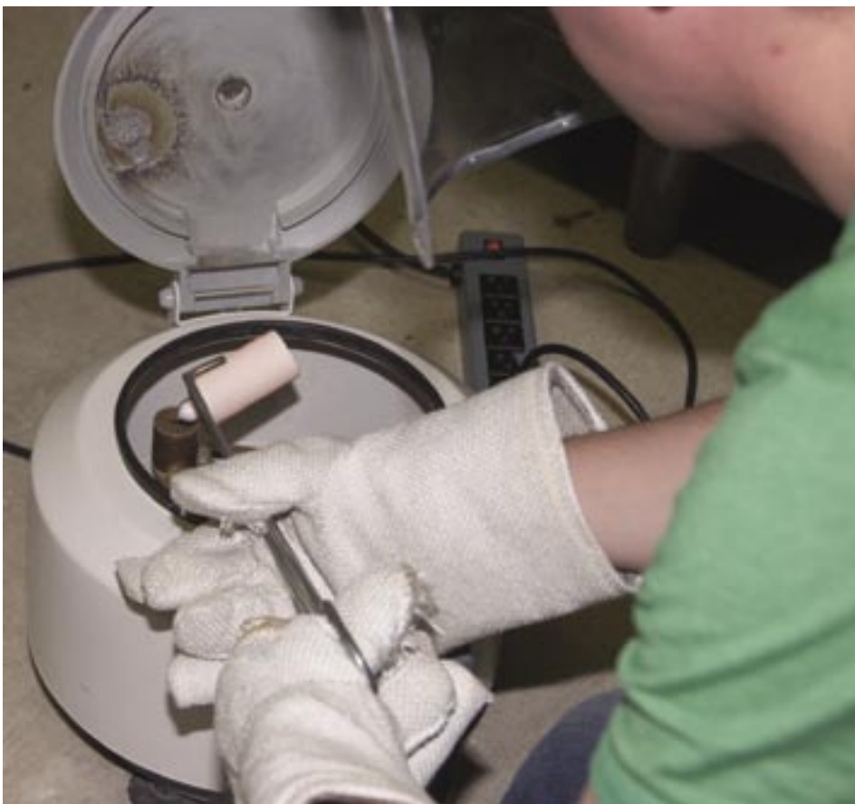
Ames Lab postdoctoral fellow Yuri Janssen pours molten alloy from a crucible into a centrifuge to separate the desired phase during a flux-growth process.
