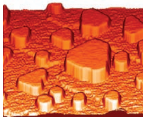
Tringides is able to grow Pb islands of five layers by using a different type of silicon surface as the substrate.
