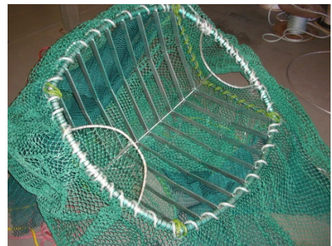
Figure 14. Fisheye BRDs incorporated into the Double Shot TED.
