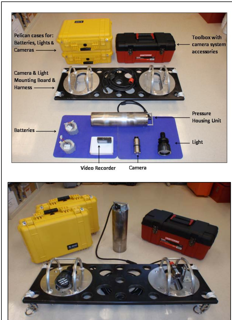
Figure 24. One of two autonomous direct observation video camera systems developed at the NWFSC with 2010 BREP funding.
