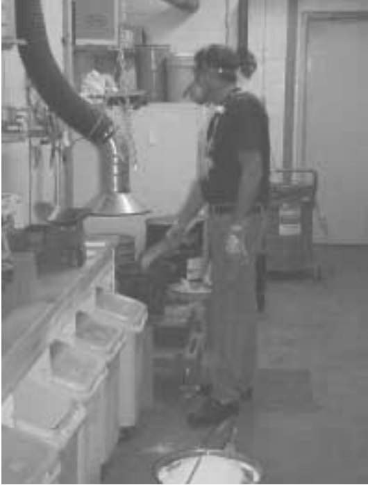
Weighing Cr(VI) pigment for colored glass production (Photo courtesy of the National Institute for Occupational Safety and Health (NIOSH)).
