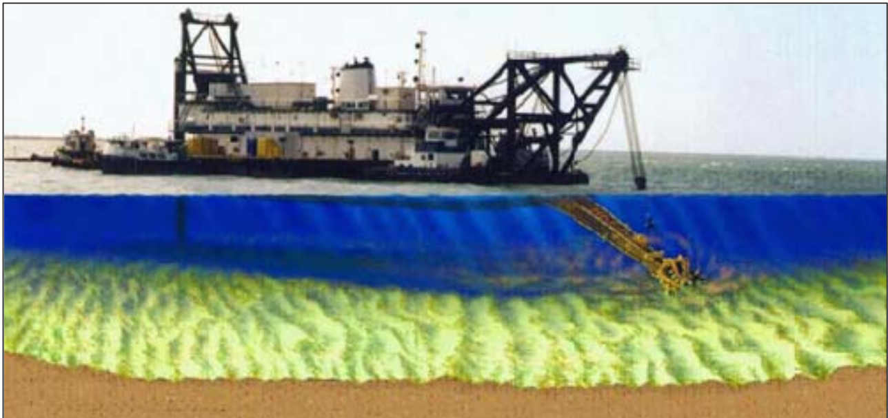
Figure 12: Cutterhead dredge graphic. (Photo/drawing:ERDC, 2007)
