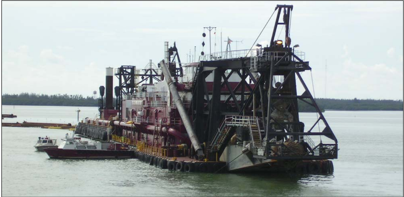
Figure 11: Hydraulic cutterhead dredge vessel. (Photo Terri Jordan)
