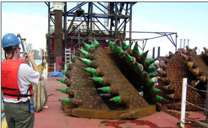
Figure 10: Typical large cutterhead Photo: Terri Jordan
