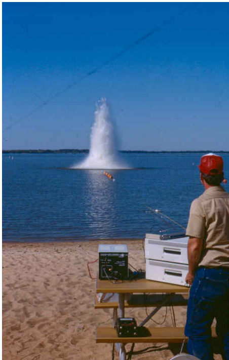
Figure 6 - Unconfined blast of seven pounds of explosives
