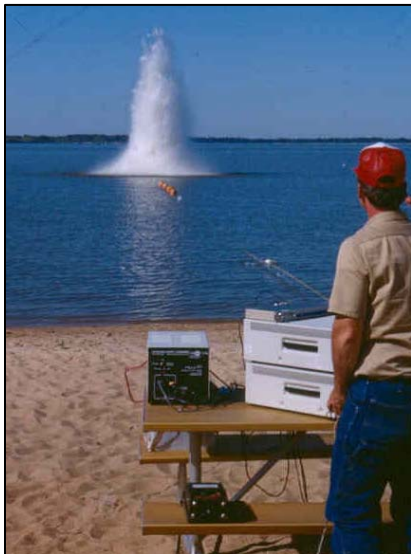
Figure 21: Unconfined blast of seven pounds of explosives.
