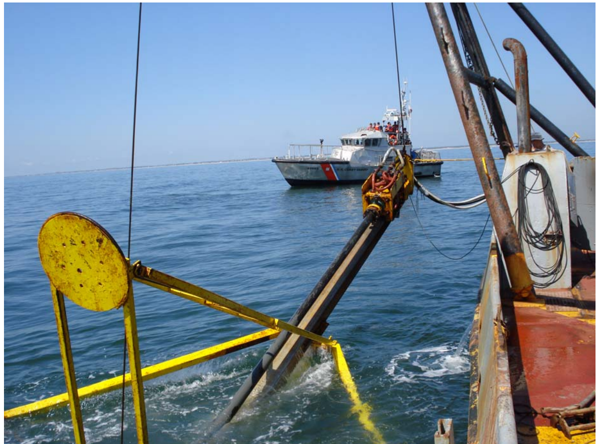
The Alpine 271 Pnuematically Powered Vibracore Unit Was Set Up To Sample 20 Ft. Cores With 3 7/8” Clear Lexan Liners.
