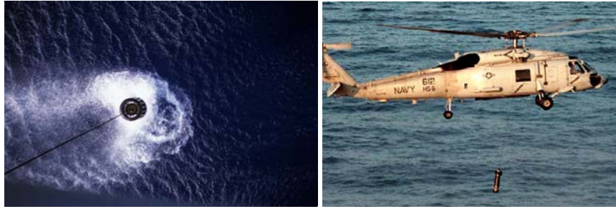
Figure C-9. AN/AQS-13 being deployed by SH-60 helicopter
