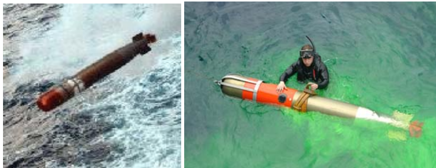
Figure C-23. MK 46 Torpedo at launch (L), and recovery (R)
