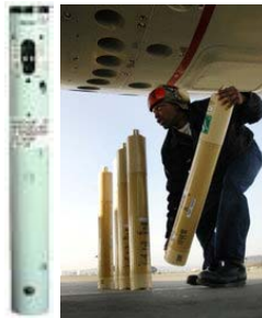
Figure C-13. AN/SSQ-53 (L); AN/SSQ-53 being loaded onto MPA (R)
