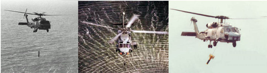
Figure C-10. AN/AQS-22 being deployed by SH-60 helicopter
