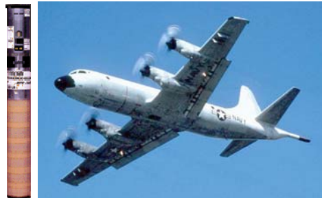
Figure C-11. AN/SQS-62 (L); MPA equipped with AN/SQS-62 sonobuoys (R)
