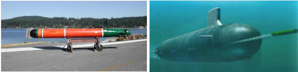
Figure C-22. MK 48/MK 48 ADCAP (L); Seawolf Class SSN launching MK-48/MK-48 ADCAP (R)
