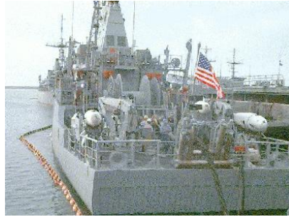
Figure C-20. Avenger Class MCM equipped with AN/SLQ-37
