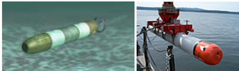
Figure C-26. MK 39 EMATT (L) and MK 30 (R)
