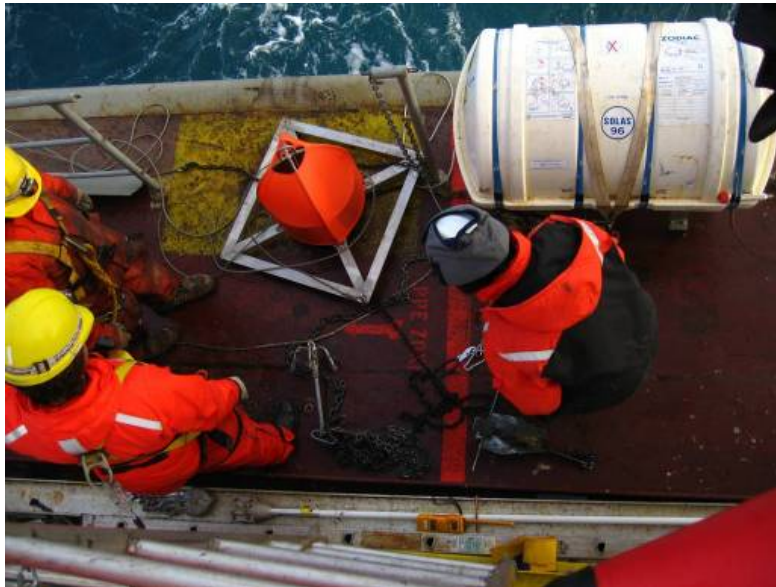
Figure 13: Photograph of a DASARb on deck after retrieval. Note the latex sock over the frame and a grapnel anchor and chain on the deck.
