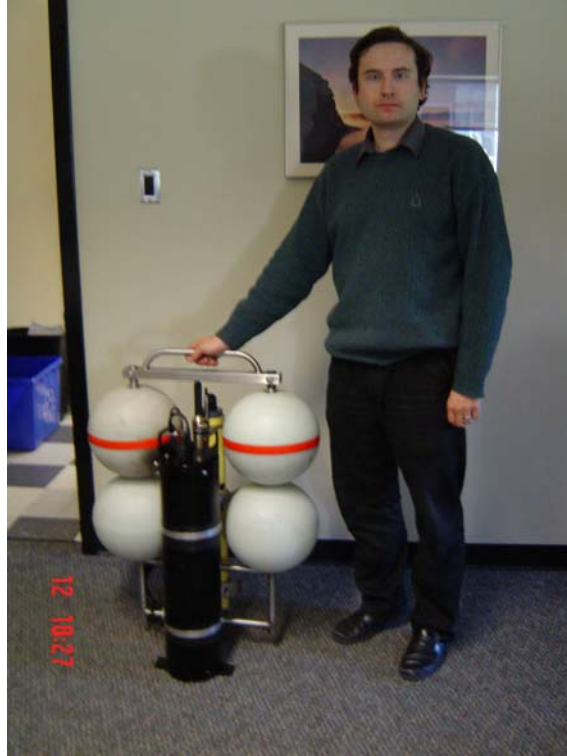
Figure 3. Ocean Bottom Hydrophone (OBH) system to be used for seismic sound source verification program, and for Chukchi Net Array program.
