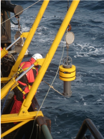
FIGURE 2. AMAR autonomous acoustic recorder for acoustic monitoring of drilling activities.
