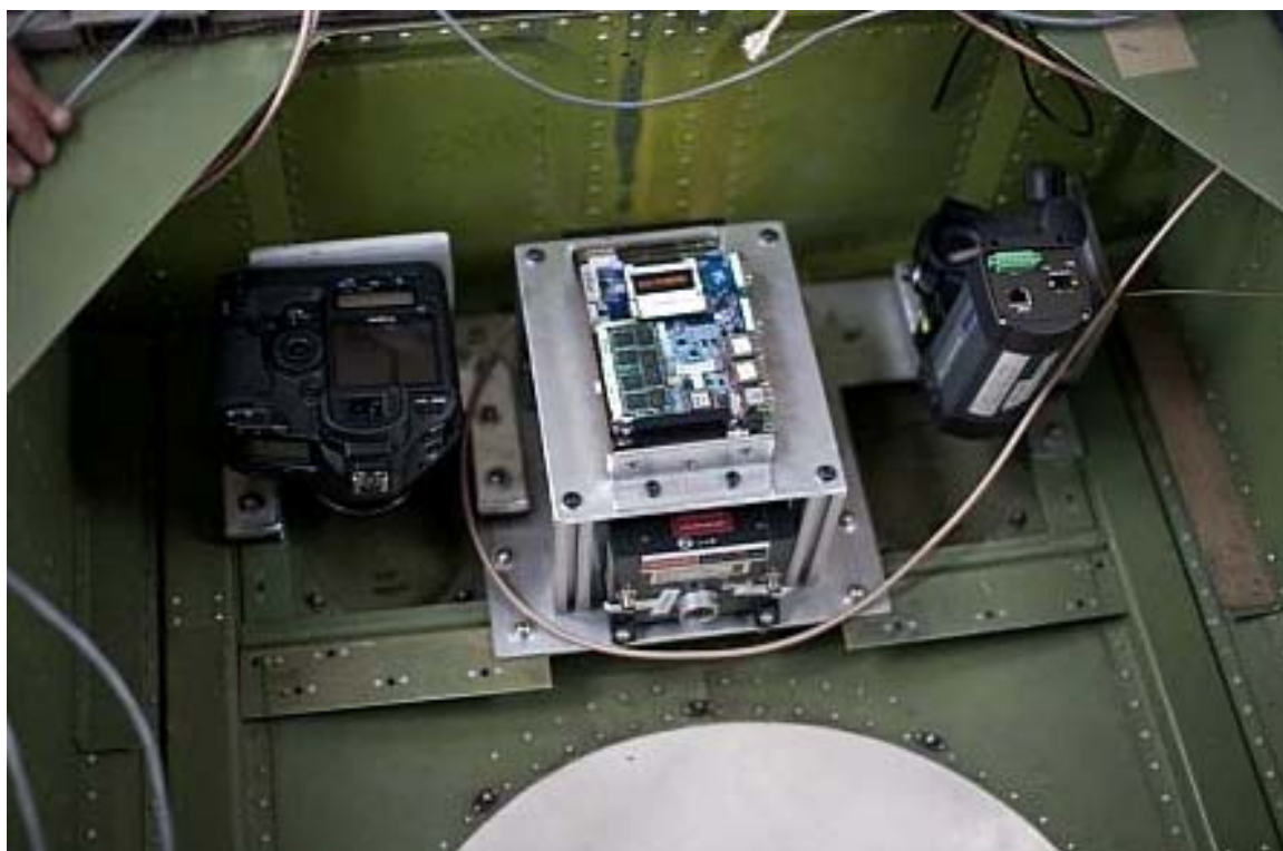
Figure 11. Camera mount and associated data storage and control devices that can be mounted as a module in a Twin Otter.
