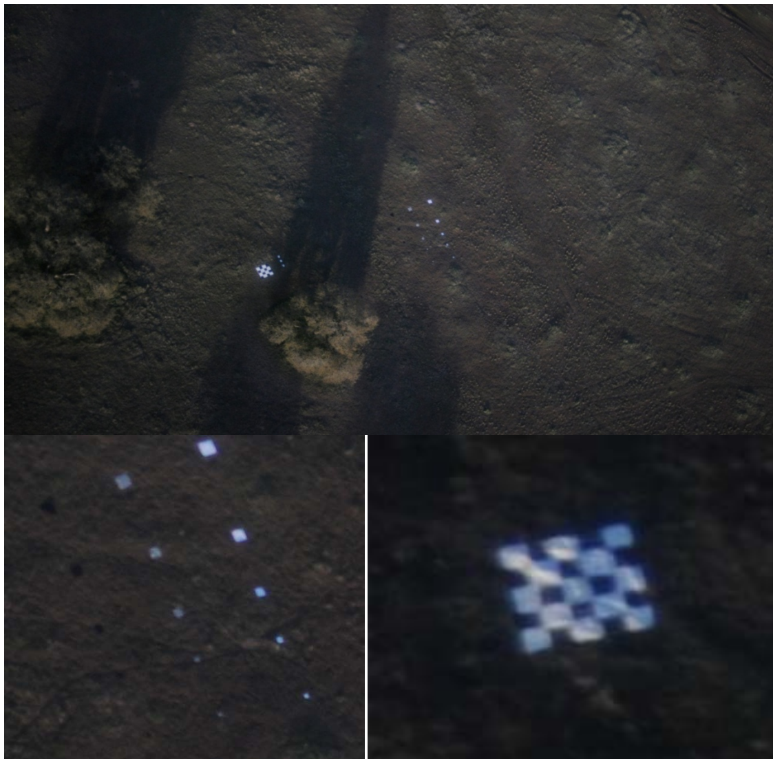
Figure 10. Photograph taken from an UAS during resolution tests at Camp Roberts, California, during December 2009. The upper photographs were taken with a 12 megapixel camera with resolution on the ground of 2.9 cm. The colored patches in the lower left photograph vary in size from 15 cm squares to 50 cm squares and are a magnified view of the upper photograph. The lower right photograph is a magnified view of a 2 m square checkerboard with each checkerboard square 40 cm by 40 cm.
