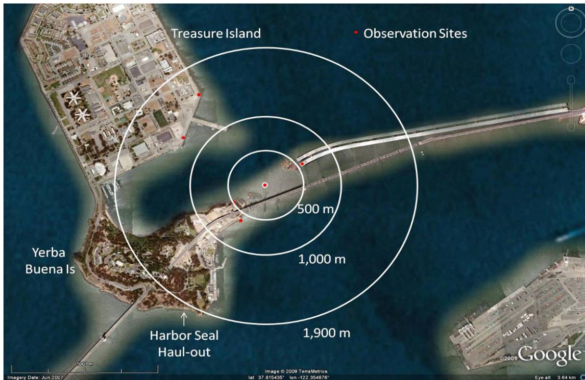
Figure 4. Map of Marine Mammal Safety Zones and Observation Sites Used During Pile Driving at Temporary Towers F and G
