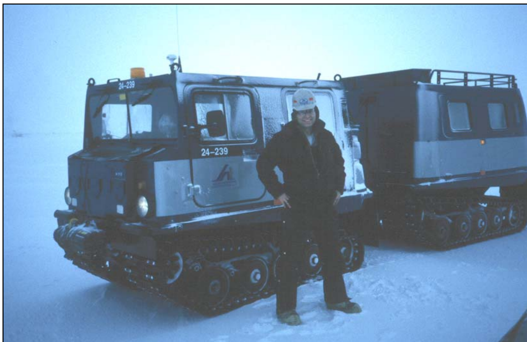
FIGURE 1.4. Hägglunds tracked vehicle and personnel carrier. Power is from a turbocharged diesel engine capable of 143 hp at 4600 rpm; total weight of the two cars is ~4536 kg (10,000 lbs).
