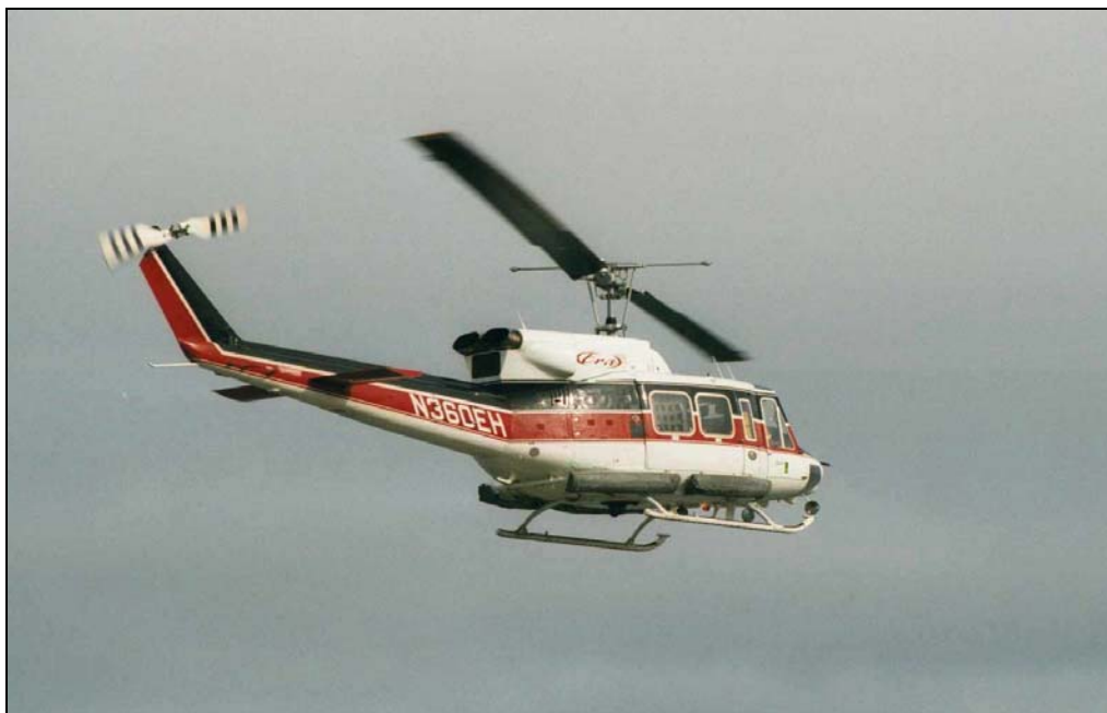
FIGURE 1.2. Bell 212 helicopter used for transportation to and from Northstar.
