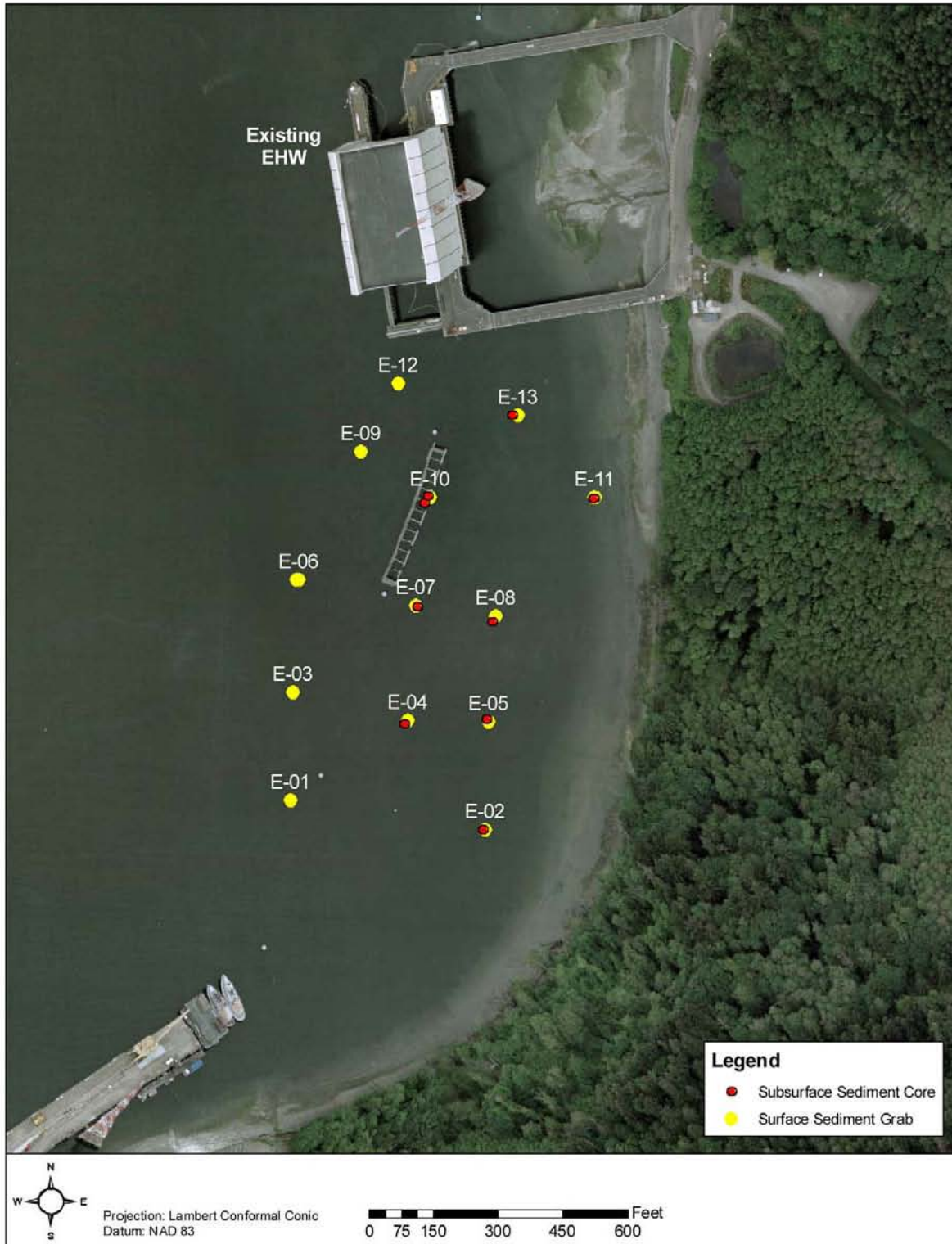
Figure 3-2. Sediment sampling locations at the site of the proposed Test Pile Program at Naval Base Kitsap Bangor (Hammermeister and Hafner 2009).
