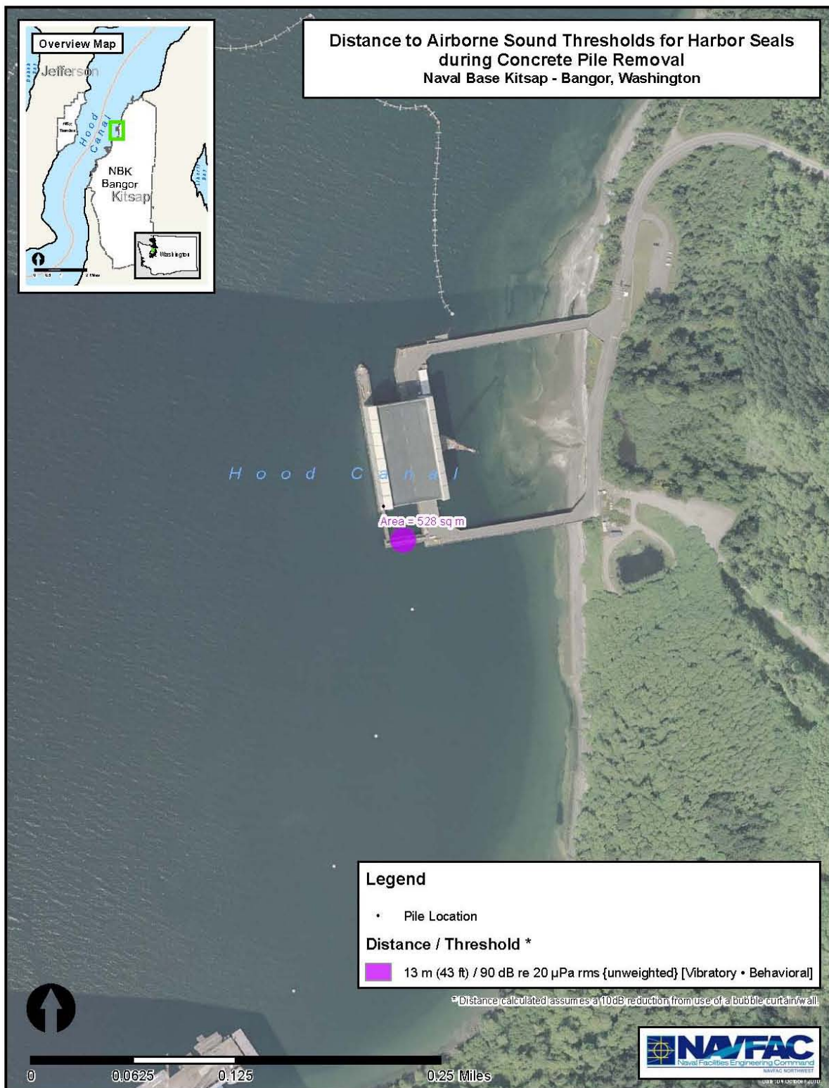
Figure 3-24 Distance(s) (m) to NMFS Airborne Sound Thresholds for Harbor Seals from a Chipping Hammer During Concrete Pile Removal
