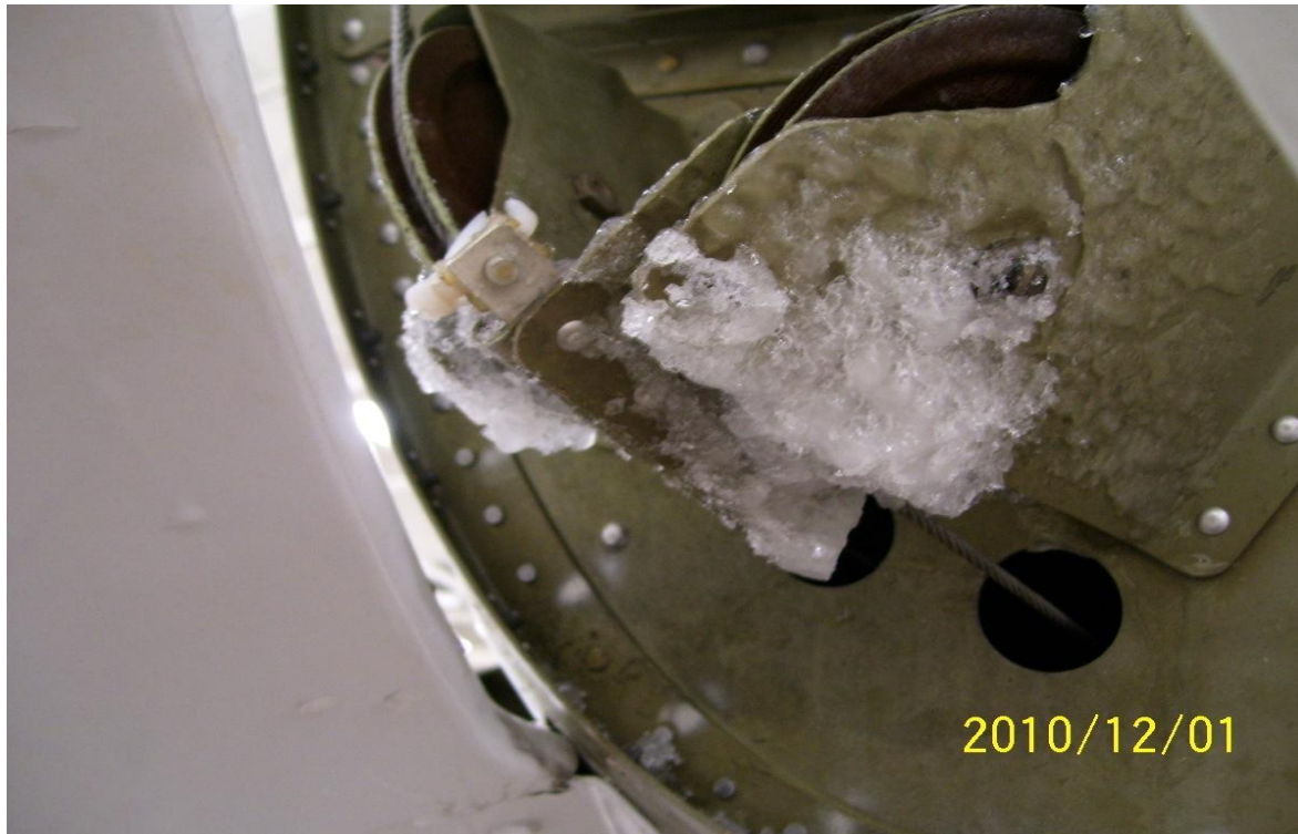
Figure 2. Ice found on the rudder boost cables and pulleys.
