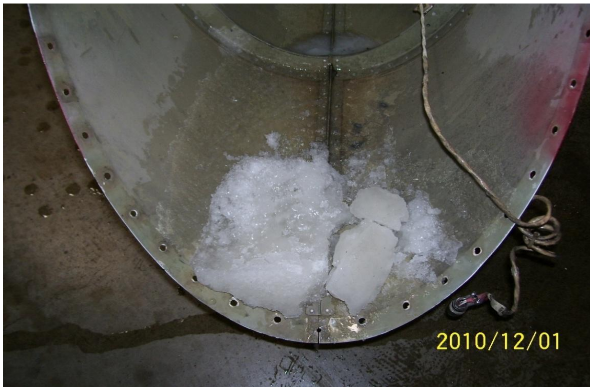
Figure 1. Ice found in the bottom of the tailcone.
