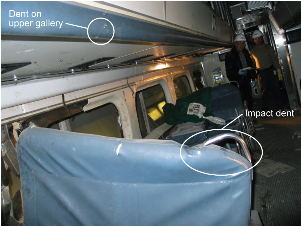
Figure 2. Seat back in front right of car 7488 showing impact dents, the location of which corresponds with the inboard edge of the underside panel of the upper-gallery level (located directly above the seat).
