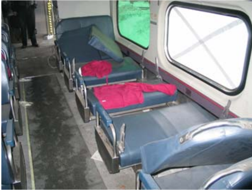
Figure 1. Exposed seat back supports in car 8548.
