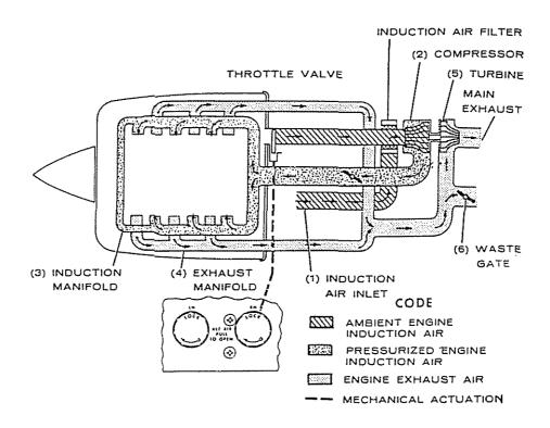
In the Cessna 421C Pilot's Operating Handbook, the manufacturer states, in part, that changes in the flow of exhaust gases into the turbine will increase or decrease the speed of the turbocharger. A leak in the exhaust system, such as the one noted at the left engine waste gate outlet flange of the accident airplane, would cause a decrease in the turbine speed, and consequently, a loss of engine power.
