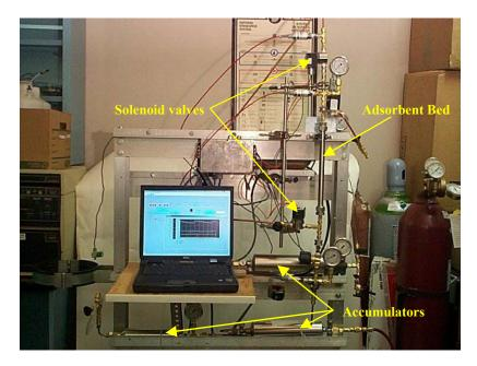
Figure 5-4. Pressure Swing Adsorption Laboratory Setup (Powertech Laboratories under an EPRI research contract).
