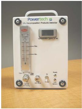
Figure 5-6 SF<sub>6</sub> Decomposition Products Detector (DPD)
