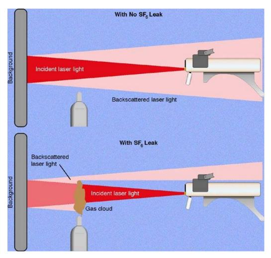
Figure 5-1. Principle of operation of the SF, Camera. Shown with and without the presence of leaking SF, [24].
