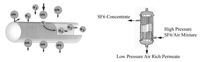
Figure 5-2 Semi-permeable membrane separation [31]
