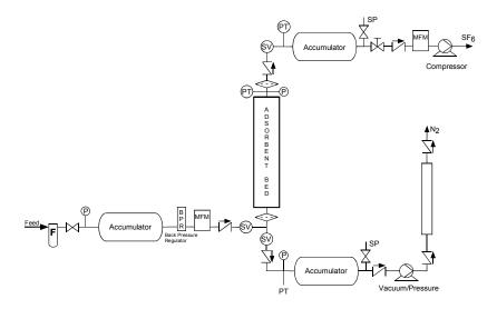
Figure 5-3. Schematic of a Simple Pressure Swing Adsorption (PSA) Apparatus. Key: sv – solenoid valve, PT – pressure transducer, P – pressure gauge, MFM – mass flow meter, BPR – back pressure regulator
