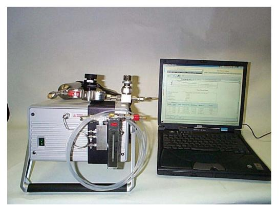
Figure 5-5 Customized Portable Gas Chromatograph [36]
