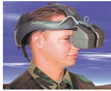
Figure 5 Kaiser Electro-Optics Video See-Through HMD Courtesy of Kaiser Electro- Optics, Inc. A Rockwell-Collins Company Used with permission
