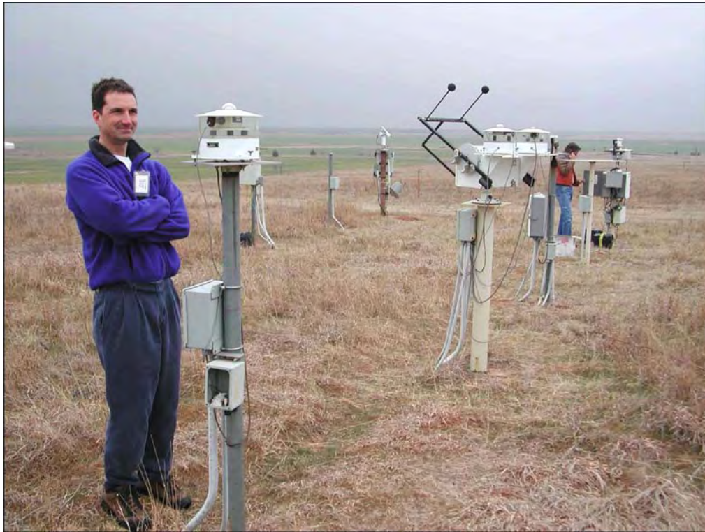
Figure 1. SIRS radiometers for downwelling irradiance measurements. (Pete Gotseff from National Renewable Energy Laboratory [NREL] inspecting the unshaded ventilated pyranometer used to measure global horizontal shortwave irradiance.)
