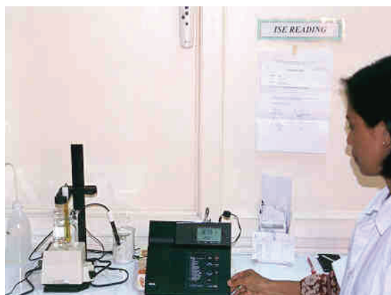
Figure 3. Ion Selective Electrodes (ISE) linked to a Thermo-Orion pH/ISE meter used by the IMA to measure cyanide ion concentrations in sodium hydroxide after reflux distillation.
