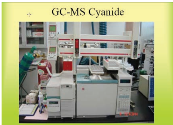
Figure 4. A gas chromatography-mass spectrometry (GC-MS) apparatus used to determine cyanide concentrations. Image provided by Dr. David Klein, Texas Department of State Health Services.
