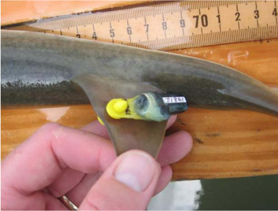
Figure 1. Acoustic transmitter attached to external fin tag with marine epoxy. Transmitters are epoxied to a rototag. Source: Poulakis et al., 2010.
