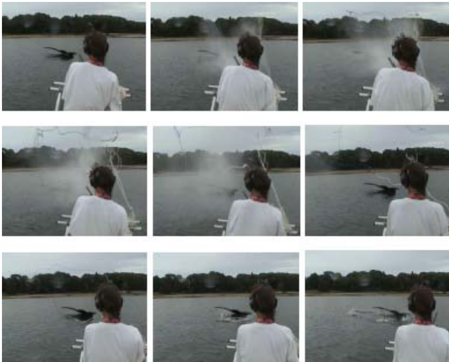
Figure 3. Successful lasso attempt on a model right whale tail during on-the-water testing of the net gun deployment system. Figure included in the initiation package sent to the ESA Interagency Cooperation Division on November 14, 2011. Photo Source: Becky Woodward, Woods Hole Oceanographic Institution.
