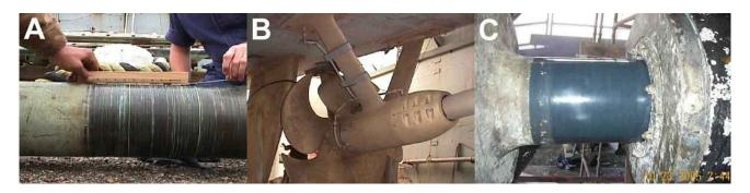
Figure 4.7 USS Ardent Propulsion Shaft Coating (A) Propulsion shaft used to suffer from significant wear during normal operation. (B) A nanostructured ceramic coating was applied to the shaft to improve wear resistance. (C) After over two years in service, no wear has been observed on the propeller shaft.<sup>[21]</sup> Courtesy of Ken Scandell, Naval Sea Systems Command Carderock Division
