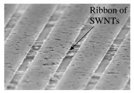
Figure 7.12 NRAM<sup>™</sup> - SWNT Non-Volatile Memory Image of SWNT memory elements Courtesy of Nantero, Inc.
