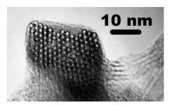
Figure 2.2 Bundle of CNTs From [9]. Reprinted with permission from AAAS.
