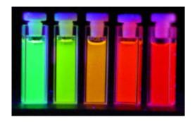
Figure 2.3 Suspensions of QDs Varying size QDs emit different light upon excitation by the same light source. Courtesy of Koninklijke Philips Electronics, N.V.
