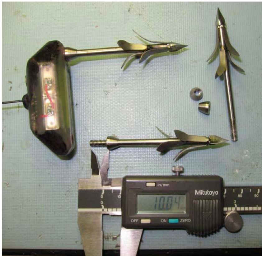
Fig. 3. Application of titanium 8-32 threaded nuts to old darts.
