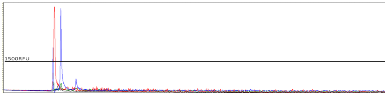
Figure 8. The LS rule firing. The Low Signal rule fires when the relative fluorescent units (RFU) are below a specified threshold which indicates that the signal intensity of the data may be too low for accurate interpretation.
