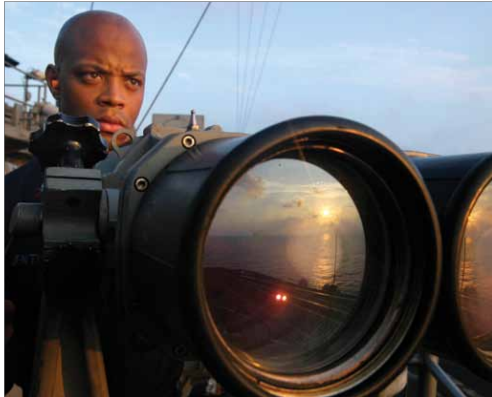
Navy lookout uses "Big Eye" binoculars to scan for surface contacts at sea, including marine mammals
