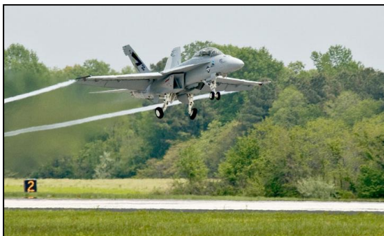
The “Green Hornet,” an F/A-18 Hornet fueled on a 50/50 blend of jet fuel and camelina-based biofuel, completed a test flight at NAS Patuxent River on Earth Day 2010.
