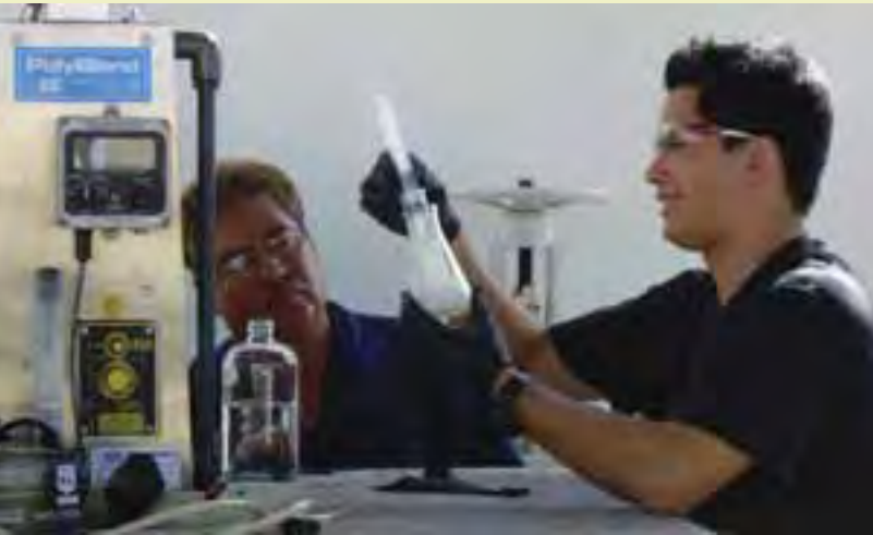
Team member Ben Fegurgur (right), conducts a quality assurance test at the Fuel Oil Reclamation Facility. These tests assure that the water can be properly discharged into the installation sewer system. In the past, the wastewater was discharged to the industrial waste treatment plant at a higher cost.
