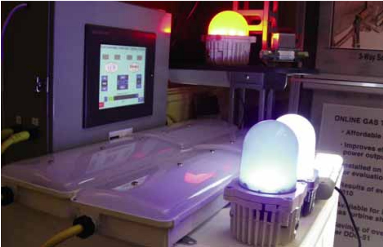
Advanced Solid State Lighting uses Light Emitting Diodes (LED) to replace conventional fluorescent and incandescent lights. LED replacements require less than 20 percent of the power of equivalent incandescent bulbs, and last close to 100 times longer. Compared to fluorescent lights, LEDs are 50 percent more energy efficient, last seven to ten times longer, and are not considered hazardous waste.
