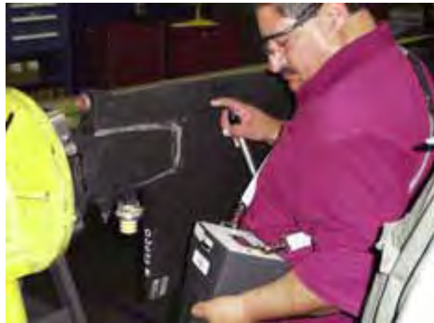
CCAD shop artisan testing the cuff of an H-60 blade.
