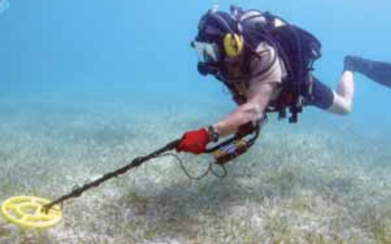
Prior to the installation of the water barrier system at the Vieques Naval Installation, a magnetometer was used to identify potential buried munitions.
