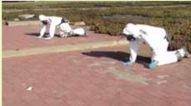
Pre-removal activity-based sampling mimicking Navy training exercises on concrete pads with asbestos-containing tiles.
