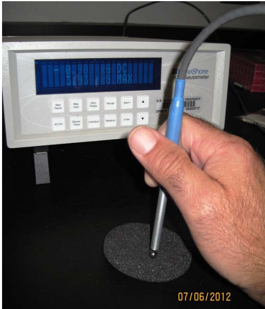
Figure 6. Gauss Meter and Axial Probe Used to Locate Magnet Surface Flux Density
