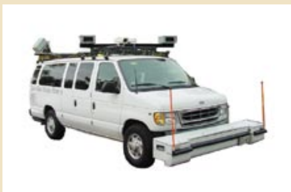
Figure 6. Photograph. New Mexico’s Department of Transportation collected data on its entire roadway system using the stereo RST van shown above.
