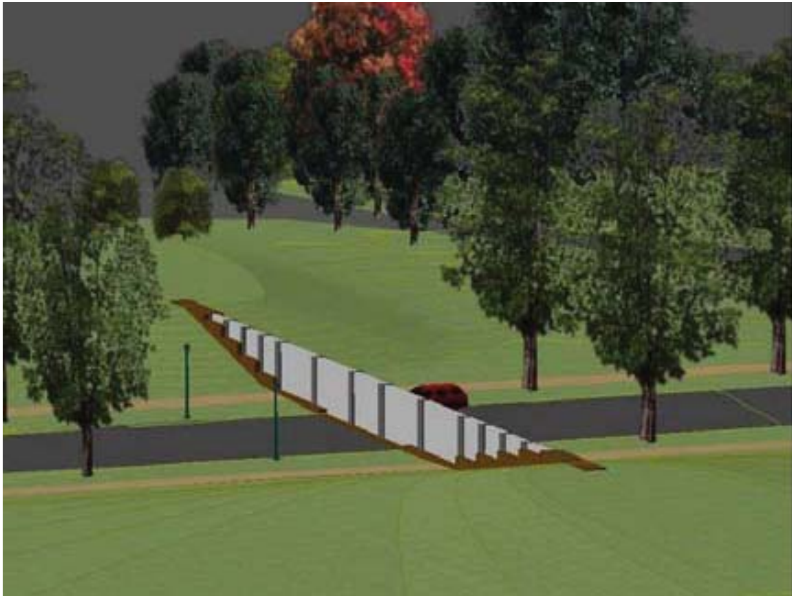
Removable post-and-panel barrier connected to permanent masonry walls and earthen berms.
