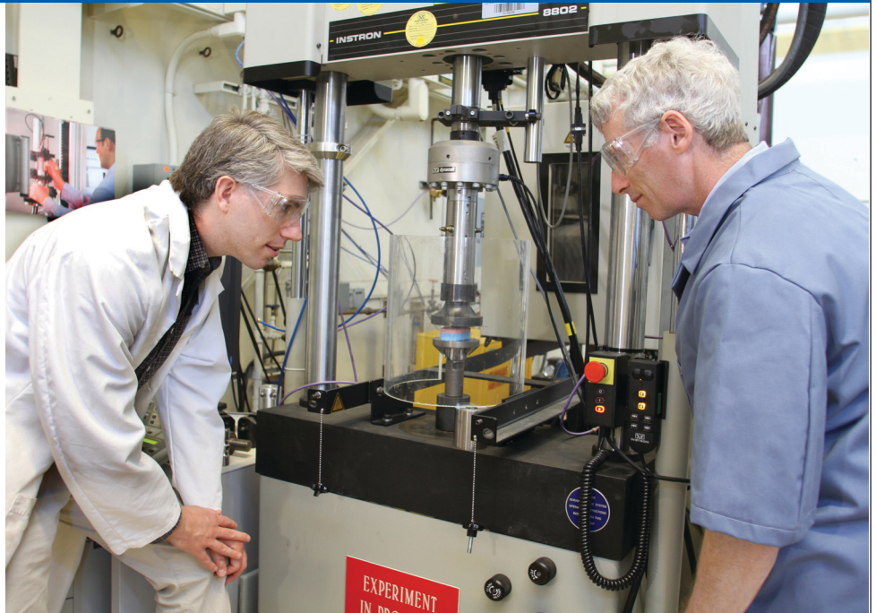
LLNL mechanical engineer Mike King (left) and physicist Willy Moss watch a compression test of a helmet pad. The pair has found a simple way to reduce the severity of traumatic brain injury from blunt and ballistic impacts.
