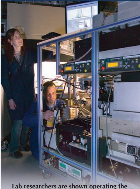
Lab researchers are shown operating the Single-Particle Aerosol Mass Spectrometry (SPAMS) system.
