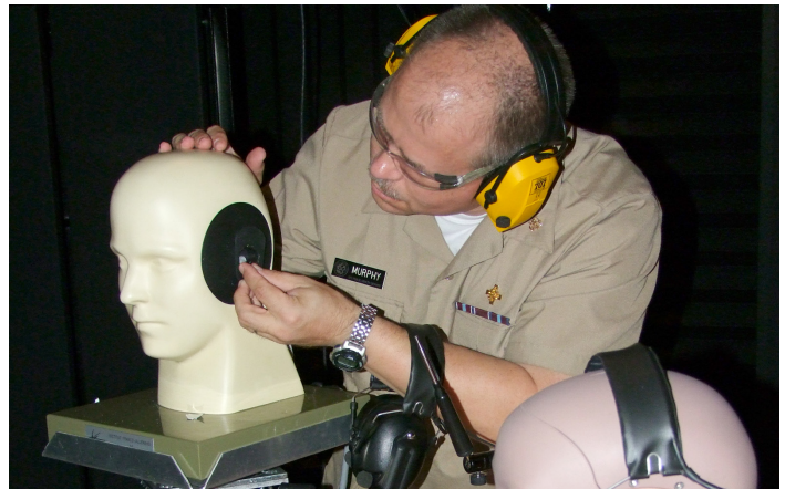
Scientist Officer CAPT William Murphy conducting tests on hearing protection devices at the US Army Aberdeen Proving Ground EAR laboratory. (US Army Photo by Ron Carty)
