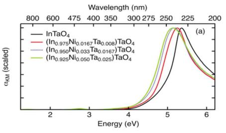
Top: A representation of the crystal structure of  $InTaO_4$  prior to doping. Bottom: Optical absorption data of  $InTaO_4$  for different levels of doping. The curves show that Ni doping does not significantly lower the band gap, which remains at nearly 4 eV. Most solar energy is found at 3 eV and below.
