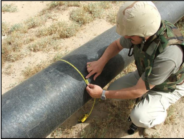
Inspector measuring pipe diameter
