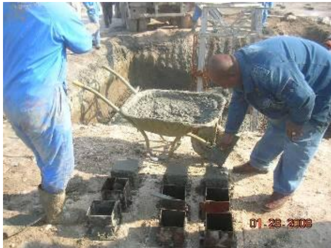
Site Photo 13. Cube test (Courtesy of the USACE)
