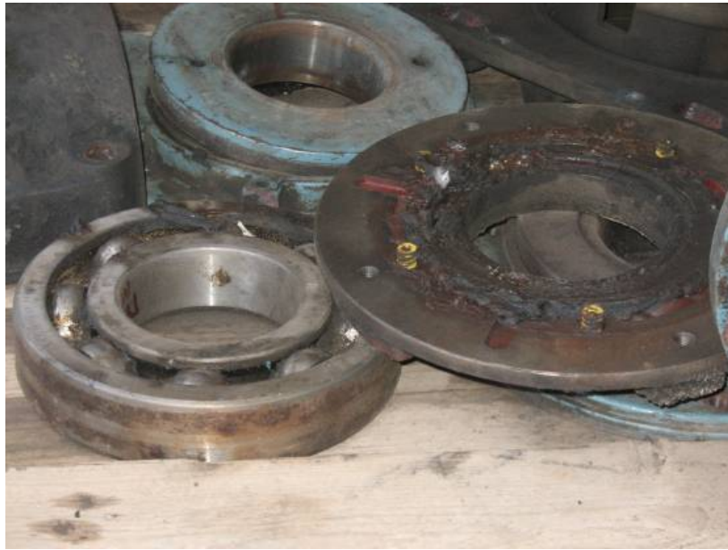
Site Photo 3. Inadequate lubrication caused bearings to fail. (10 June 2007)
