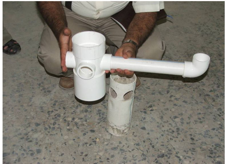
Site Photo 15. Contract specified wastewater pipe connection method
