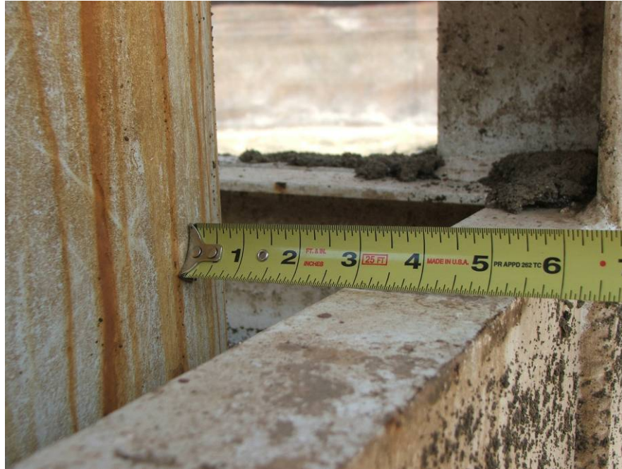
Site Photo 6. Main shaft was positioned approximately 2 7/8 inches from the static frame.
