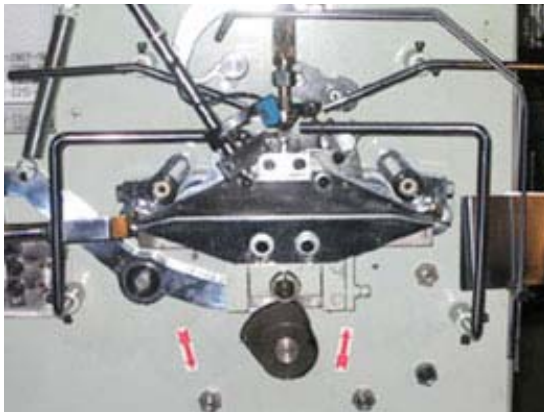
Detailed view of wire entering formation process. Hanger is formed.
