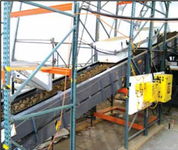
Painesville Soil Being Processed Through Soil Segregator
