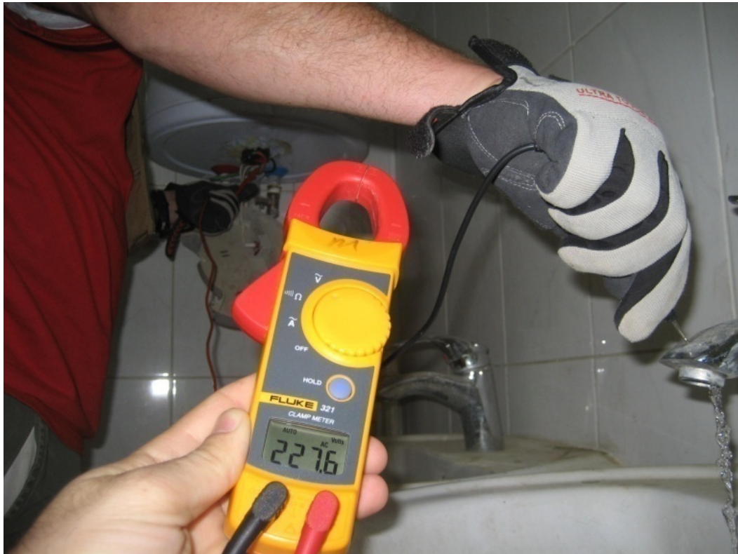
Figure 3—Photograph of voltmeter reading in water stream
