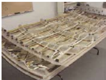
Figure 6. Mockup of an Aircraft Fuselage Panel with a Variety of 10 Foot Wiring Harnesses and Connector Types. Each Harness has Multiple Documented Insulation and Conductor Defects.
