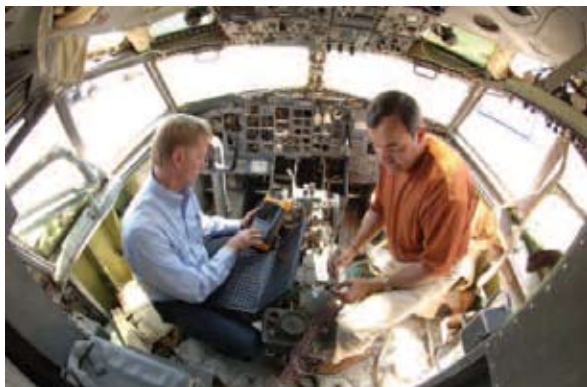
Figure 1. Inspection of Aircraft Wiring Systems.
